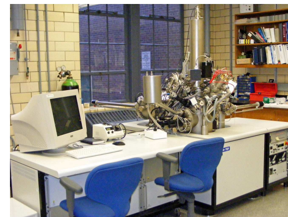
ION-TOF ToF-SIMS IV - the first 3-column ToF-SIMS IV
